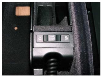
When the setting is "locked", the interior and outside trunk release button inputs are ignored.
